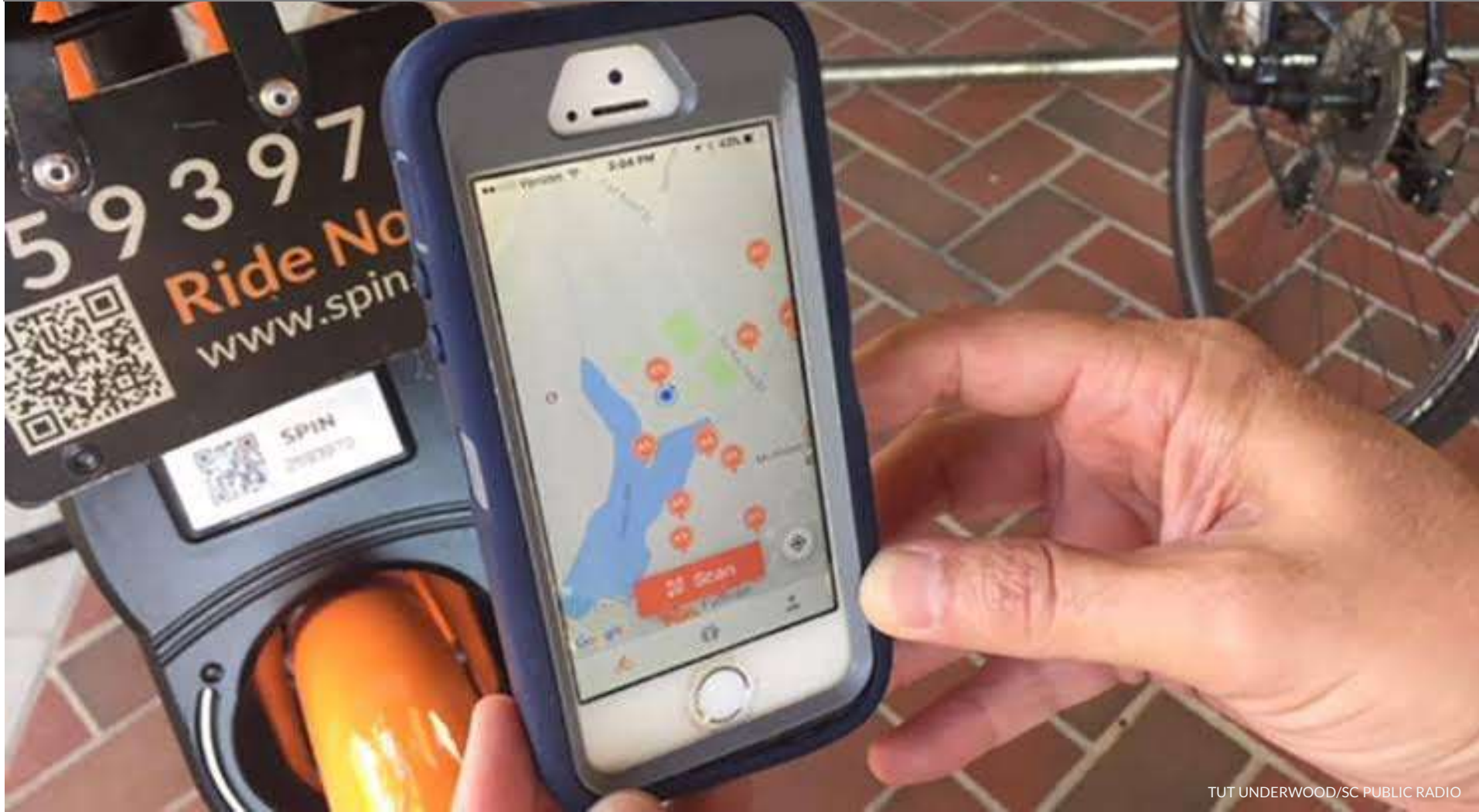
Dockless shared vehicles: Download app, find vehicle, scan QR code, unlock, ride.
